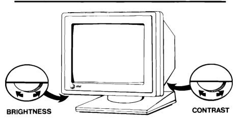
1 Turn the display screen's brightness and contrast controls all the way forward.
