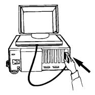
2 Insert and screw in the end of the display screen cable to the connector on the rear right of the main unit.
