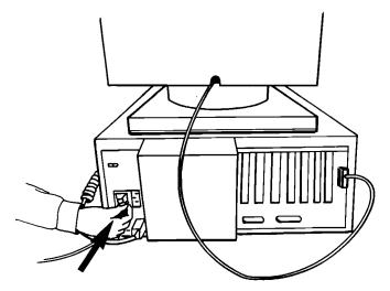
3 Connect the female end of the power cable to the INPUT AC socket on the rear of the main unit.
