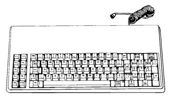
6 Place the keyboard in front of the main unit. Two adjustable legs are available on the underside of the keyboard. Use them to raise the keyboard as necessary.
