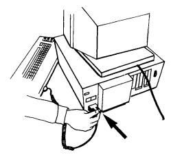
1 Insert and screw in the end of the keyboard cable into the keyboard socket on the lower left rear corner of the main unit.
