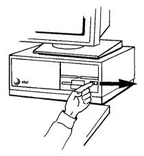
1 Unlock the diskette drive door by moving the drive door lock switch to the right. When the drive door is locked, the red square to the right of the lock button is exposed. When the drive is unlocked, the red square is covered. Your computer may not be equipped with door locks. If so, continue to the next step.
