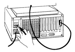
2 Turn on the computer. The on-off switch is located above the power cable socket on the rear of the main unit.
